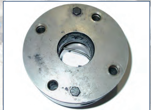
Packing with damaged internals
