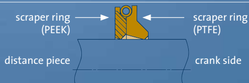
Special geometry of the scraping edges of the BOSS oil wiper packing
