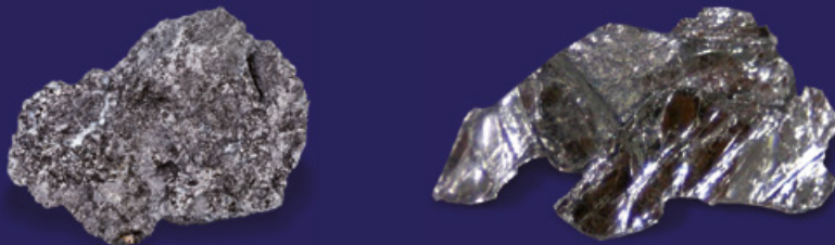
Graphite (left) and molybdenum disulfide (right) as efficient dry lubricants
