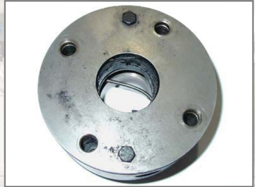
Packing with damaged internals
