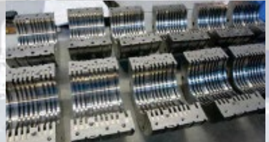
Seal casings of STASSKOL SDW20 (high pressure version)
